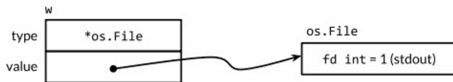
Figure 7.2. An interface value containing an *os.File pointer.
