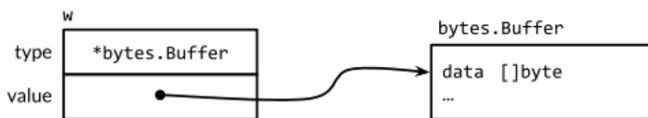
Figure 7.3. An interface value containing a *bytes.Buffer pointer.
